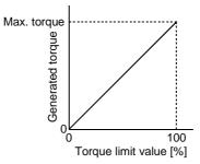
A relationship between the applied voltage of the analog torque limit (TLA) and the torque limit value of the servo motor is shown below. Generated torque limit values will vary about 5% relative to the voltage depending on products.
